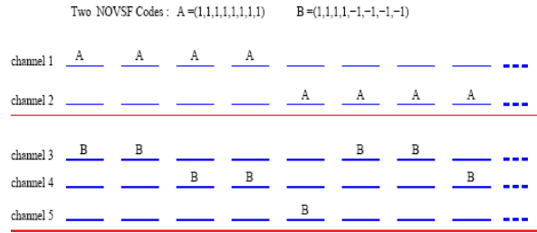
Figure shows Two NOVFS codes are shared in time among at least five different channels.
